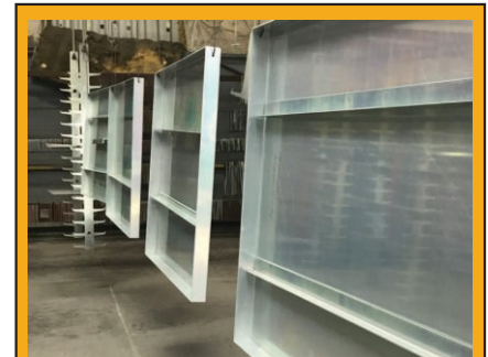
3M VHB Tapes are fully cured allowing stiffeners to be pre-taped prior to assembly.
